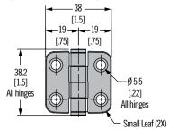
Recommended mounting holes: tapped M4 (8-32) thread or Ø 4.5 ± 0.1 (1.77 ± .004) thru All hinges
