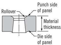
Mounting holes may be drilled, punched, or cast.
