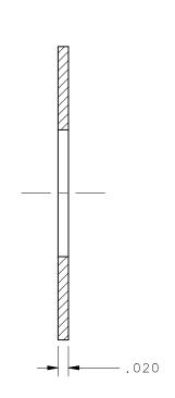
NOTE: TO SELECT PROPER STUD SIZE WHEN SEALING WASHER IS REQUIRED - ADD THICKNESS OF WASHER (.020) TO TOTAL THICKNESS OF MATERIAL TO BE FASTENED.
